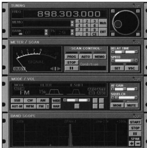
The PC-based PCR-1000 Control Software Set to Monitor a BlackBerry Transmission
