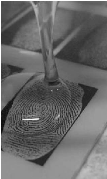
Creating a Fake Gelatin Finger to Bypass a Biometric Fingerprint Sensor (Photos obtained from http://www.itu.int/itudoq/itu-t/workshop/security/present/s5p4.pdf and modified)
