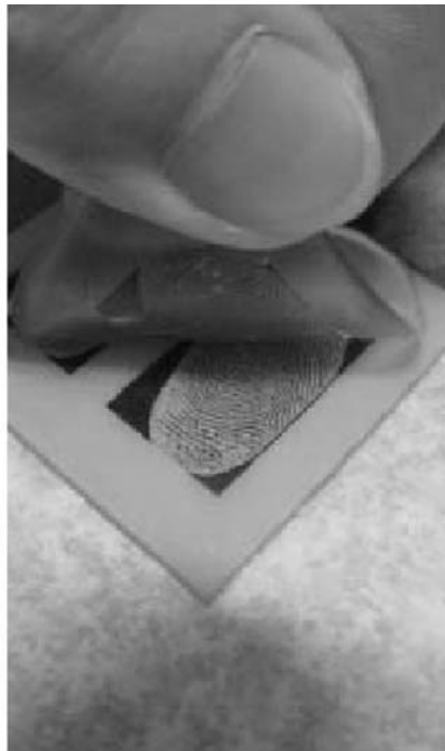
Creating a Fake Gelatin Finger to Bypass a Biometric Fingerprint Sensor (Photos obtained from http://www.itu.int/itudoq/itu-t/workshop/security/present/s5p4.pdf and modified)
